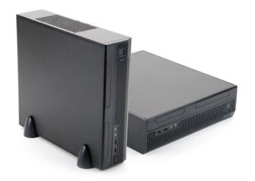
VeryPC Flex is a slimline small form factor (SFF) PC with the capability to mount a VESA compatible monitor using its optional bracket. The bracket not only saves desk space, but is adjustable in all directions: tilt, rotate, swivel and height. Every Flex comes with a lockable cable shroud and compact stand feet for stably orienting your desktop in a slim mini-tower configuration.
